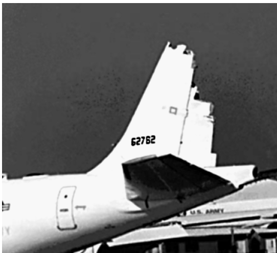
Fig. 4 Example of structural failure caused by flutter.
